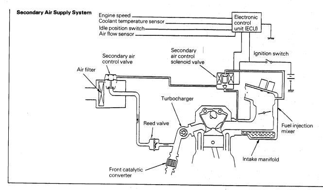
The reed valve supplies secondary air into the front catalytic converter for the purpose of promoting oxidation of exhaust emissions during the engine warm-up operation, the engine-hot-start operation and the vehicle deceleration.
