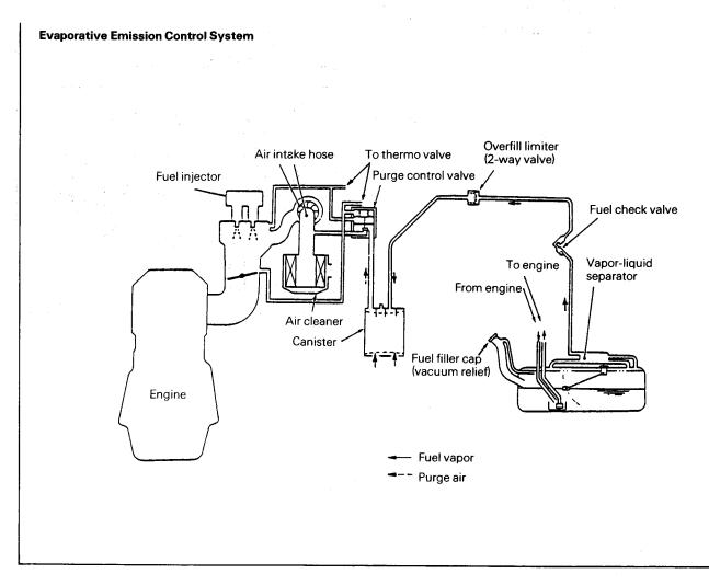
The purge control valve is kept being closed at idling to prevent vaporized fuel from entering into the air intake hose for positive control of high idle CO emissions which is particularly a problem under high ambient temperature condition. And once the pressure difference between the turbocharged and the throttle ported-pressures exceeds the pre-set value, the purge control valve is opened.
