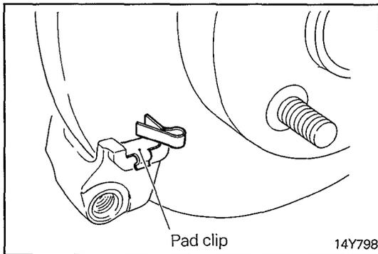
(15) Install the pad clip to the caliper support.
