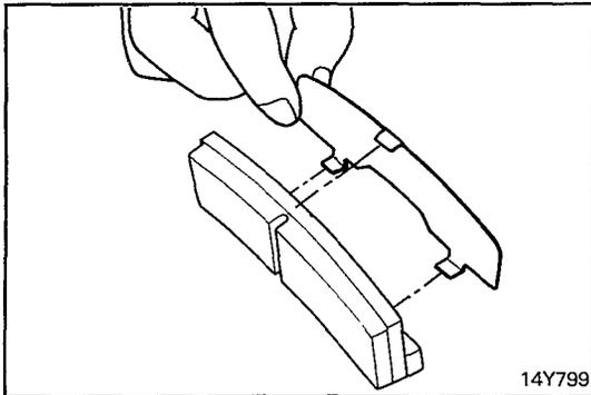
(16) Install with shim pawl engaged with the pad assembly as illustrated.
