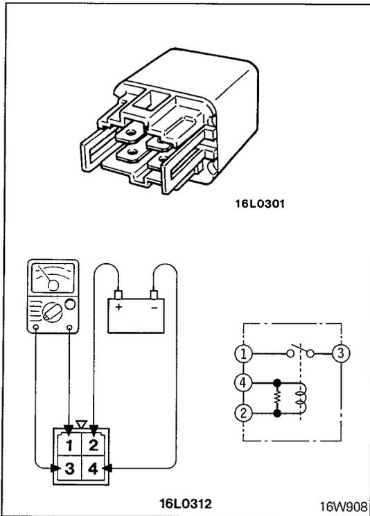
(2) Check continuity between terminals when the battery voltage is applied to the terminal 2 and the terminal 4 is grounded.
