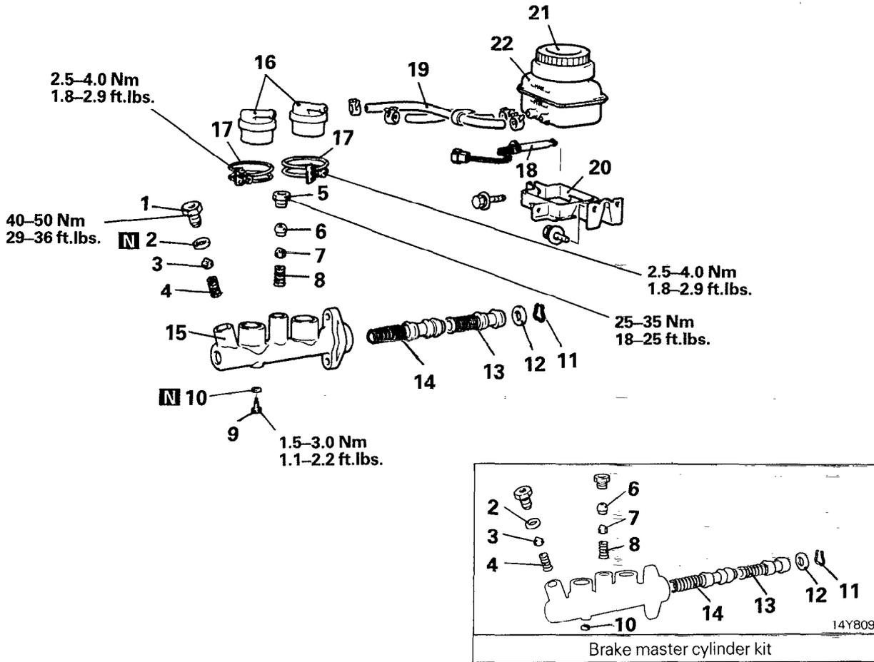
**Brake master cylinder disassembly steps**
