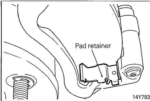
(14) Install the pad retainer to the caliper support.
