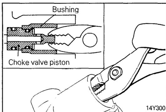
**17. REMOVAL OF BUSHING / 18. CHOKE VALVE PISTON**
