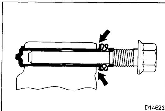
**6. APPLICATION OF GREASE TO BUSHING**
