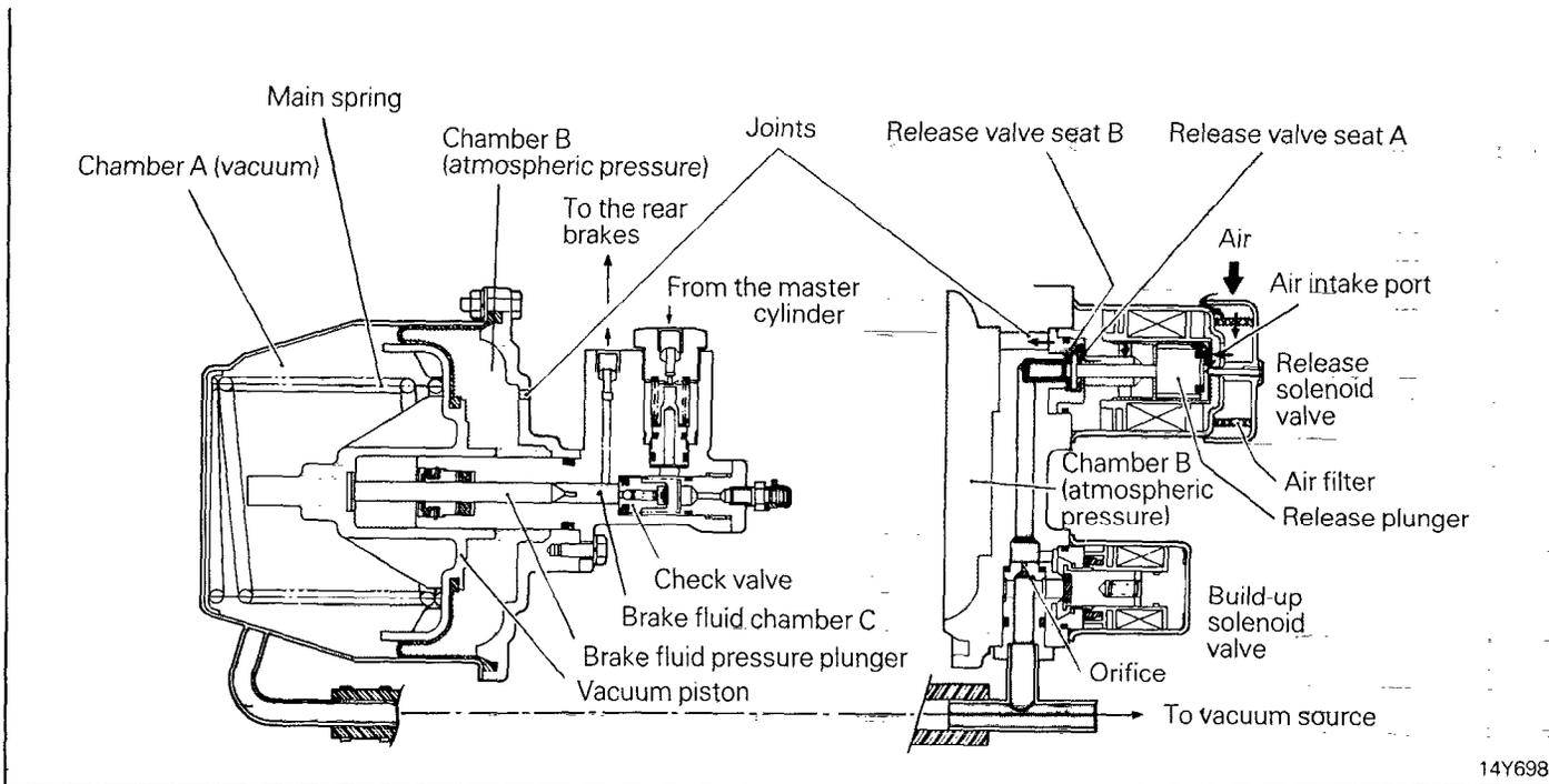
2. Slow restoration of the brake fluid pressure for the rear brakes to a normal level
