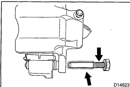
**1. APPLICATION OF GREASE TO SLIDE PIN**
