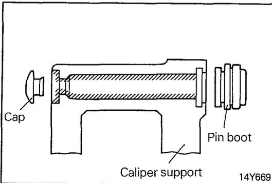
**8. APPLICATION OF GREASE TO CAP / 7. PIN BOOT**
