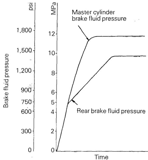
When the brake fluid pressure reaches 4,903 kPa (711 psi), the stepped diameter piston will press the cut-in spring upward, and contact the plug. The brake fluid will pass only through the V-shaped groove, thus limiting the rate of increase of the brake fluid pressure to the rear brakes.
