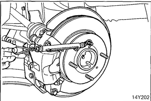
(19) Measure the brake drag by starting the engine, maintaining the brake pedal in the depressed position for approximately 5 seconds while the vehicle is not moving, and then rotating the disc ten revolutions in the forward direction and using a spring balance to measure the brake drag in the forward direction.
