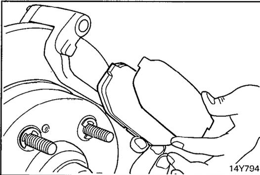
(15) Install the inner and outer shims to the pad assembly.
